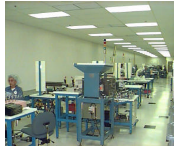
Class 10,000 clean room
